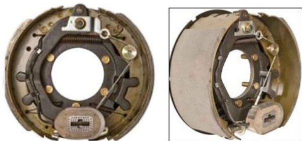
Brake assm. 12-1/4" x 5" electric. 5 bolt mounting
